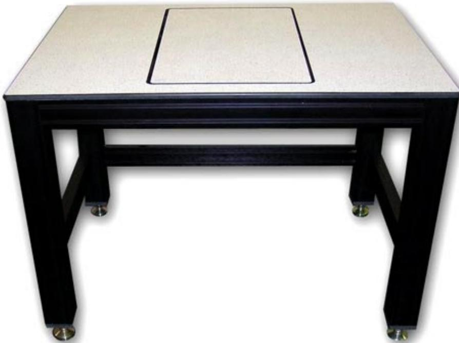
The Vistek Series 2500 Vibration Isolation Table (VIT 2500) is an exceptionally rigid, elegant, table built with extruded anodized aluminum shapes. Designed for the microscope user, vibration isolation is provided only where you need it, which is beneath the microscope and recessed within the table. This makes it possible to perform critical microscopic observations and use the work surface at the same time, without any workflow interruption.
