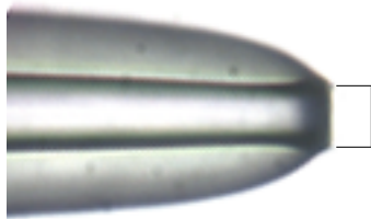
10 micron ID tip pulled with HPLC tubing on P-2000/F
